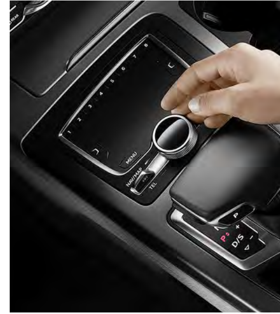
Audi Q7 which features haptic feedback controls.
